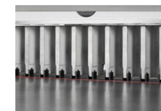
Backgauge rakes with plastic gliders treat the table surface with care
